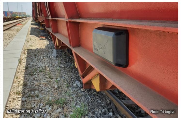
The RailBlazer application for rail freight provides fleet owners, railway companies and shippers with instant insights into a freight car's location, condition and functionality. Through the hybrid communication system, precise tracking, including the positioning of wagons in the train formation and marshalling yard, is possible.
