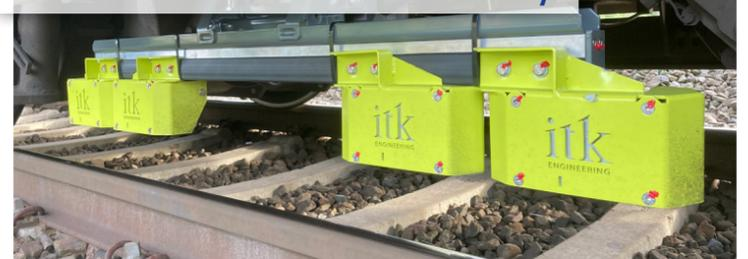
The position of a vehicle is determined by changes in the electromagnetic field
